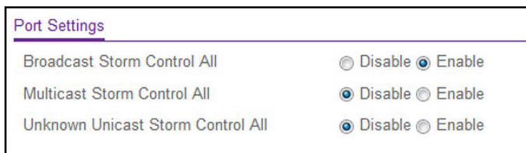
The following three controls provide an easy way to enable or disable each type of packets to be rate-limited on every port in a global fashion. The effective storm control state of each port can be viewed by going to the port configuration page.
