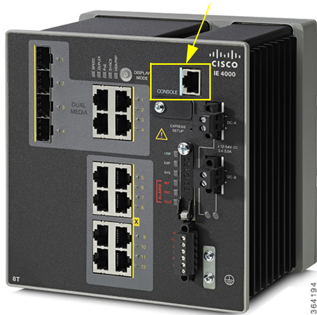
Figure A-2 Connecting the Console Cable
