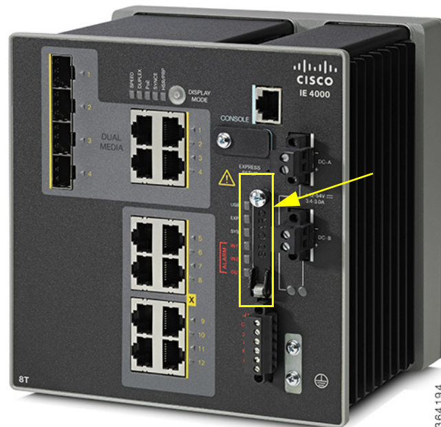
Figure 2-1 Installing the Flash Memory Card in the Switch
