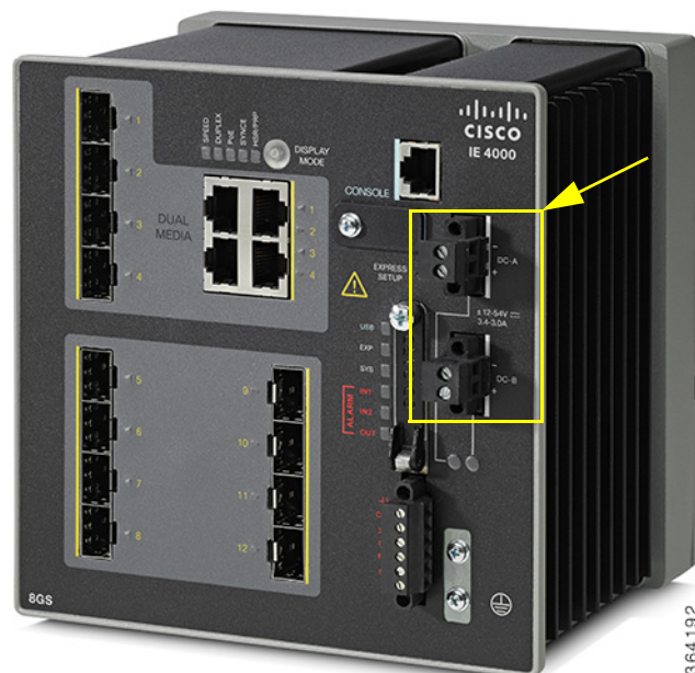
Figure 2-5 Removing the Power Connectors from the Switch
