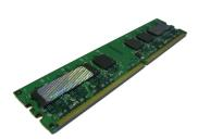
16GB, DDR3, 1333MHz, 240-pin DIMM
