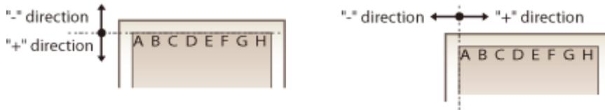
In the example shown below, to shift the print position 5 mm upward and 1.7 mm rightward, "-5.0 mm" is set in <Offset Y> and "+1.70 mm" is set in <Offset X>.
