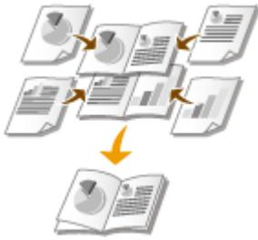
You can print two pages of a document on both sides of paper and then fold your printed pages in half to make a booklet. The printer driver controls the print order in such a way that the page numbers are correctly arranged.
