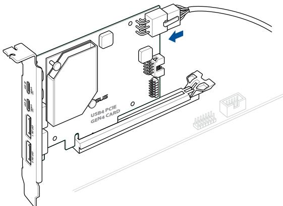
6. (optional) Connect the DisplayPort cable to the USB4 PCIE GEN4 CARD's DisplayPort IN port (A) and to the DisplayPort on the motherboard's I/O port (B).
