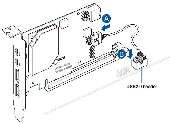
5. Connect the 6-pin PCIe power connector from the PSU to the USB4 PCIE GEN4 CARD.
