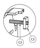
ii. Slide item C1 down the front slots of item A1 to the correct height and tighten items C2.
