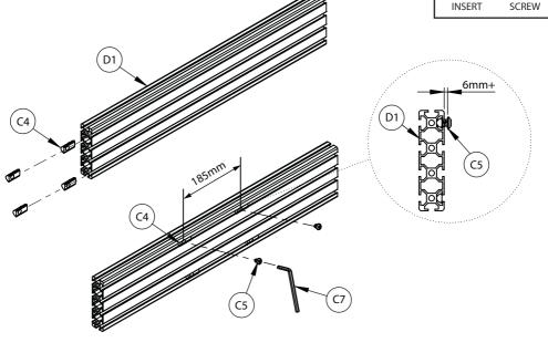
iii. Hook item D1 onto item C1 and fix with in place with item C5.
