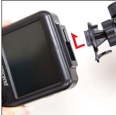
2. Thoroughly clean the area of the windshield you wish to mount the dashcam. If possible, mount it in the middle of the windshield and close to the height of the rear-view mirror for the best field of view.
