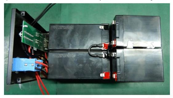
Step 2 : Install the two batteries into the battery box as shown in the figure
