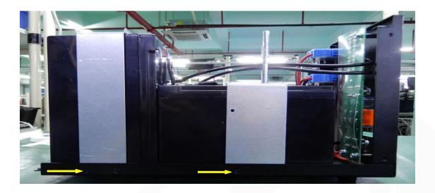
**Step 4 :** Connect the battery cable, pay attention to the red connection and the black connection.
