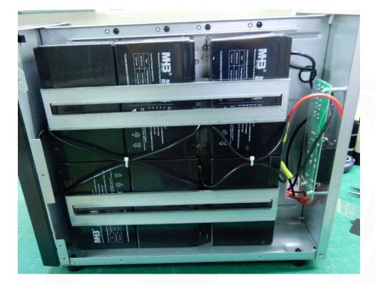
**Step 4:** Switch to the other side, use the wires connect the batteries follow the picture.
