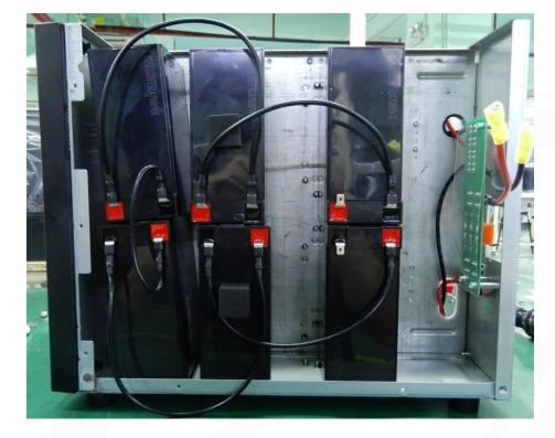
**Step 1:** Use the wires connect the batteries follow the picture.
