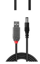
Power DC equipped devices from a USB port Use a 5V USB port to power external (max. 3A/5V) drives or peripherals USB 2.0 Type A connector 2.1mm Inner / 5.5 Outer DC Power connector For use with compatible DC devices Length: 1.5m 10 Year Warranty Black Lindy Adapter Cable USB A male - DC 5.5/2.1 mm male. Cable length: 1.5 m. Connector 1: USB A, Connector 2: DC, USB version: USB 2.0, Connector gender: Male/Male, Product colour: Black
