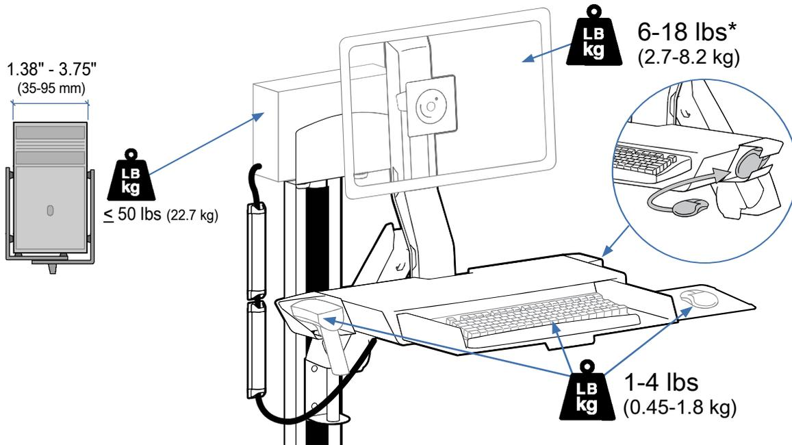
\* The Combo Arm can be modified to mount displays up to 20 lbs (9.1 kg), however display lift and tilt motion will not be possible if this option is chosen. Refer to special instructions on page 13.
