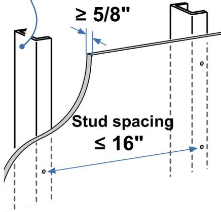
Requires minimum material thickness of 5/8" (16 mm).
