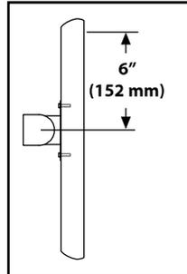
Mounting height assumes there is a 6" (152 mm) distance between the center of your monitor mounting holes and the top of the screen. If your distance is smaller, you should increase mounting height accordingly, if your distance is larger, you should decrease your mounting height accordingly.
