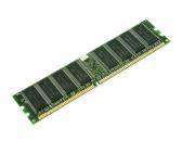
16GB DDR5, 288-pin DIMM, 4800MHz, Unregistered (unbuffered) HP N02929-001. Internal memory: 16 GB, Internal memory type: DDR5, Memory clock speed: 4800 MHz, Memory form factor: 288-pin DIMM
