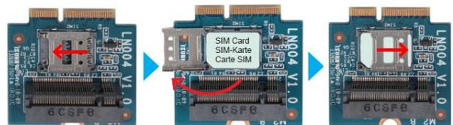
4. Please install the LTE adapter board into the M.2 E-Key slot interface as shown and affix it by tightening the screw with bolt firmly.
