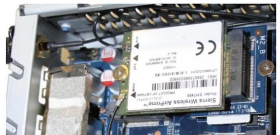
The installed riser card with additional LTE/4G card (top view) and SIM card (hidden). The pre-installed WLAN card and WLAN antenna must be removed before.
