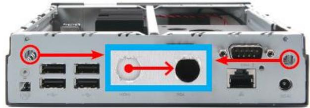
3. When installing a nano SIM card, please push the cover to the side and lift it, then carefully insert the SIM card.
