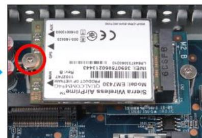
7. Take out the two antenna cable connectors and remove the locks and protective sleeves. Then connect them to the LTE module.
