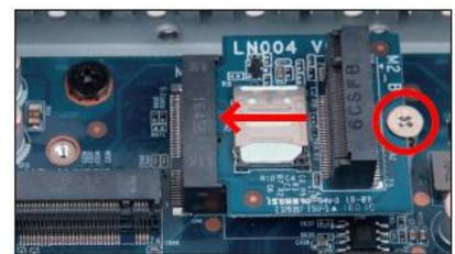
5. Please apply the bolt and tighten it firmly.
