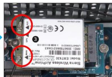
8. Install the antenna cable connectors through the appropriate opening at the back of the chassis. When leading the cable connector through the opening, check the socket alignment and only push horizontally. DO NOT turn or twist the cable. Should any difficulties occur, make sure the surface is clean. Finally, check the alignment again and carefully apply more force.
