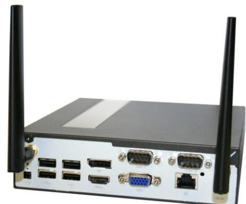
DL10J with installed cellular antennas.
