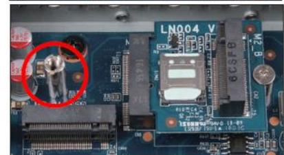
6. Please install the LTE module in the daughter-board, then tighten the screw with bolt firmly.
