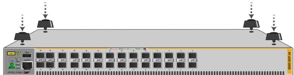
7. Turn the switch over again and place it on a flat, secure surface (such as a desk or table), leaving ample space around the unit for ventilation.
