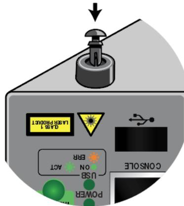
6. Push the feet firmly into holes on the base of the switch so that the rivets lock the feet in place as shown in Figure 12 on page 24
