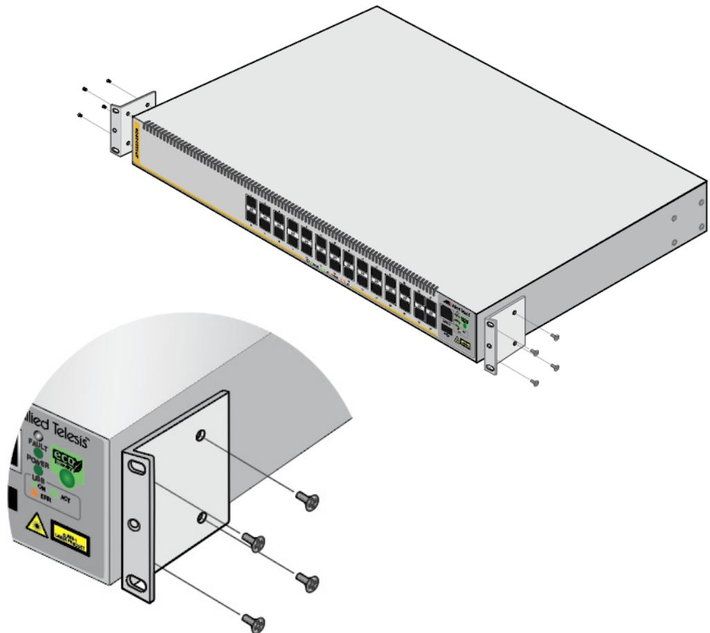
4. Mount the switch in a 19-inch equipment rack using four equipment rack screws (not supplied).
