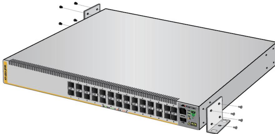
3. While another person holds the switch at the wall location, use a pencil to mark the wall with the locations of the two screw holes for each bracket. (Figure 19).
