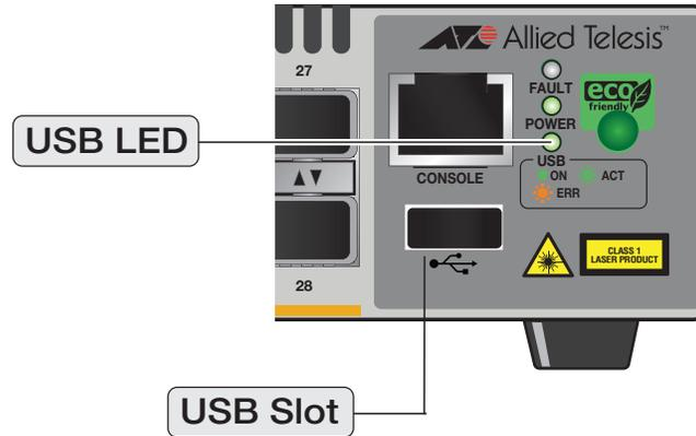
The USB LED indicates whether the USB slot has a USB inserted, or is reading or writing to the USB device. Table 4 describes the functions of the USB LED.
