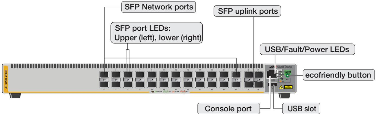
Figure 3 illustrates the back panel of the AT-x220-28GS Gigabit Ethernet Switch.
