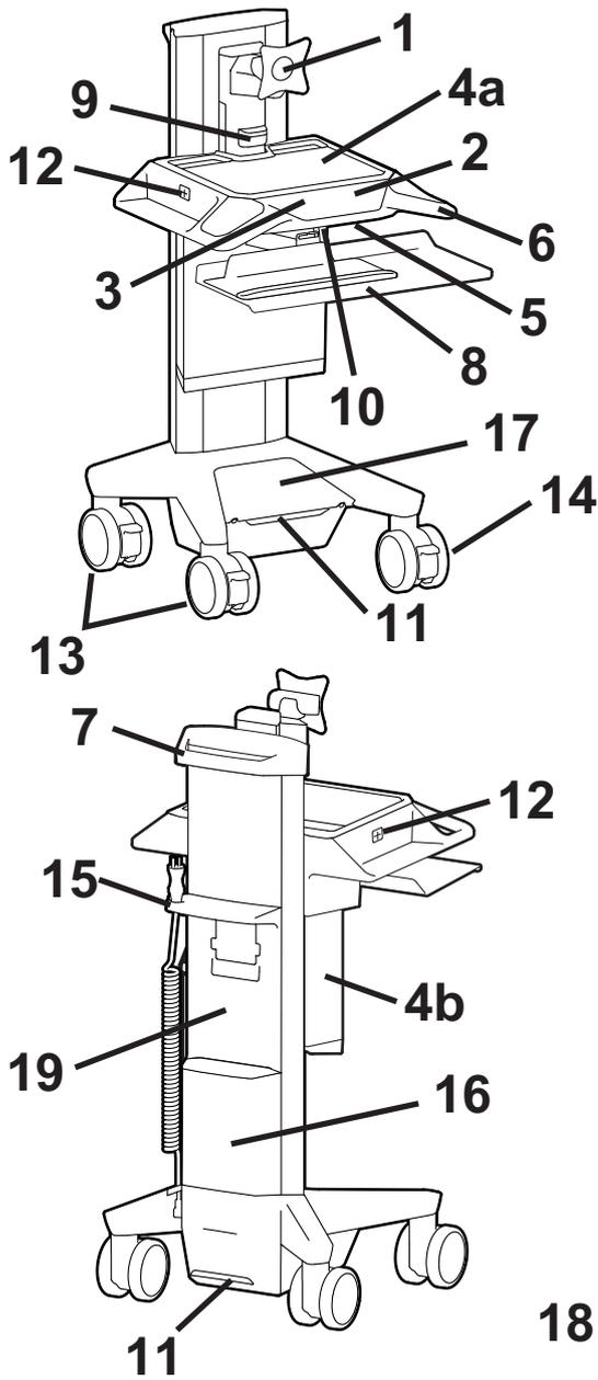
1. LCD Mount for LCDs or Tablet PC's with 75x75 or 100x100mm Mounting Interface and Provides Extension, Tilt, Pan, and P/L Rotation
