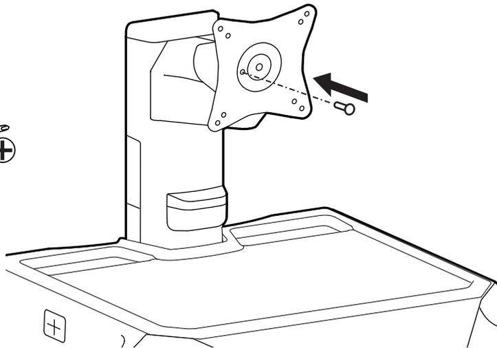
Monitor Lift Lock for monitors weighing 14 - 20 lbs (6.35-9.1 kg)
