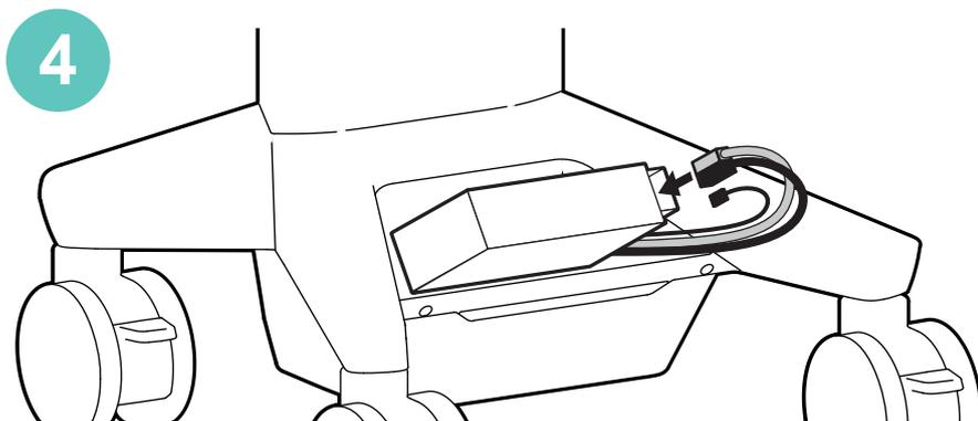
**!** CAUTION: Do NOT pinch battery cables. Pinching will cause damage to cables.
