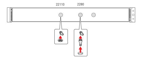
**5.** Insert your M.2 SSDs into M.2 slots at a 30-degree angle.
