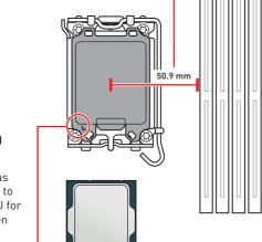
Distance from the center of the CPU to the nearest DIMM slot.
