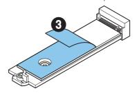
**4.** If you install 2260 SSD, remove the screw from the M.2 plate and then install supplied EZ M.2 Clip kit on the M.2 plate. Skip this step if you install 2280 SSD.
