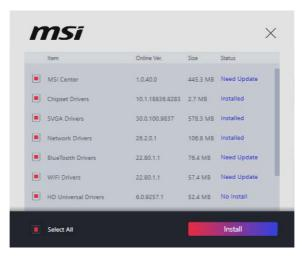
5. Check the Select All checkbox in the lower-left corner and click Install to install MSI Center and drivers. The installation progress will be shown at the bottom.
