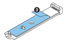
Remove or exchange the screws according to your SSD length. Skip this step, if you install 2280 SSD.
