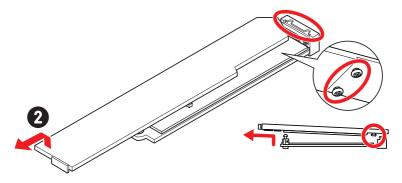
3. Remove the protective films from the M.2 thermal pads on the M.2 plate.
