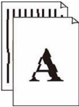
Lines Are Misaligned/Distorted
