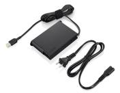
Lenovo GX20Z46271. Purpose: Laptop, Power supply type: Indoor/outdoor, Input voltage: 100 - 240 V. Product colour: Black. Cable length: 1.68 m, Width: 118 mm, Depth: 77 mm. Quantity per pack: 1 pc(s), Cables included: USB Type-C, Package type: Box
