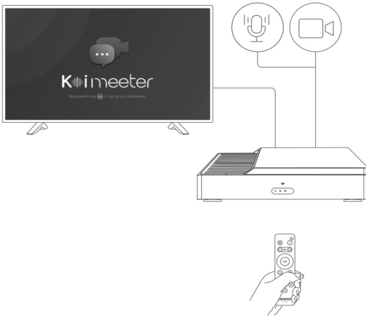
Connect the USB camera and microphone.
