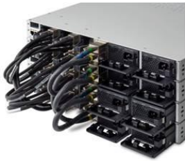
Figure 4. Cisco Catalyst 9200 Series Switch Stacked Units
