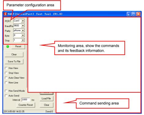
Set the parameters (baud rate, data bit, stop bit and parity bit) correctly to ensure reliable RS232 control.
