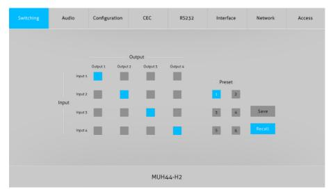
Use the 4x4 button grid on the page to set which inputs are directed to which outputs. For example, clicking the button on the Input 1 row and Output 1 column, directs input 1 to output 1.
