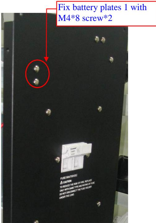
Fix battery plates 1 with M4\*8 screw\*2
