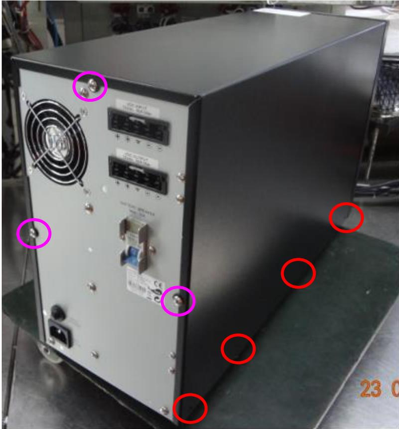
1. As shown: put back the rear panel to the machine.
