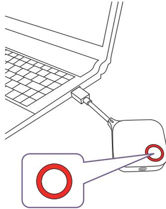
3. When the InstaShow button is ready to present, the LED indicator will turn green. Press the Present key when the LED indicator turns green.
