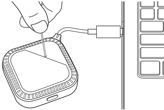
4. The InstaShow Button LED will begin quick flashing red (flash red twice every second) for 10 seconds, then light up static red for 15 to 20 seconds, indicating that the InstaShow Button is resetting.
