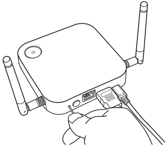
3. The InstaShow Host LED will begin quick flashing red (flash red twice every second) for 10 seconds, then light up static red for 15 to 20 seconds, indicating that the InstaShow Host is resetting.
