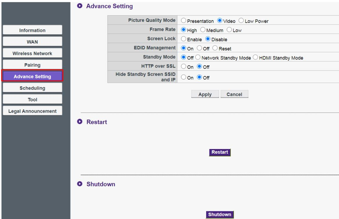
You can change mode to **Presentation** mode, **Video** mode, and **Low Power** via **Picture Quality Mode**. The default mode is **Presentation** mode. Be aware that after the firmware is upgraded to v2.01, the default mode will be changed to **Video** mode. The mode set by **Picture Quality Mode** in web management is the default mode next time when the InstaShow host restarts. That is, if the mode is **Video** mode and is switched to **Presentation** mode by the InstaShow button while playing
