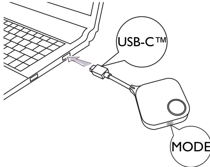
2. When the InstaShow Button is connected to the laptop, the LED indicator of the InstaShow Button will flash red. The InstaShow Button is in pairing mode, waiting to pair with your InstaShow Host.
