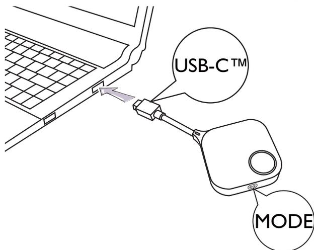
2. When the InstaShow Button is successfully connected to the laptop, the LED indicator of the InstaShow Button will blink red.
