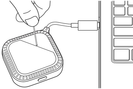
3. The InstaShow Button LED will begin quick flashing red (flash red twice every second) for 10 seconds, then light up static red for 15 to 20 seconds, indicating that the InstaShow Button is resetting.
