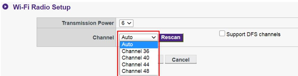
In cases when the broadcast of a presentation is unstable or choppy, due to interference to the wireless connection between the InstaShow Host and InstaShow Button from other wireless devices in the area, users can switch the **Channel** by pressing **Rescan**. By pressing **Rescan** the InstaShow Host will switch to the wireless channel with the best performance and least interference at the time.
