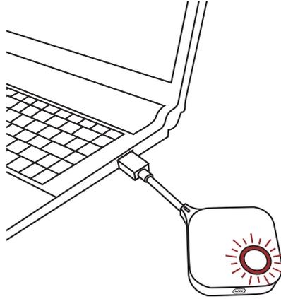
3. When the InstaShow button is ready to present, the LED indicator will turn green. Press the Present key when the LED indicator turns green.
