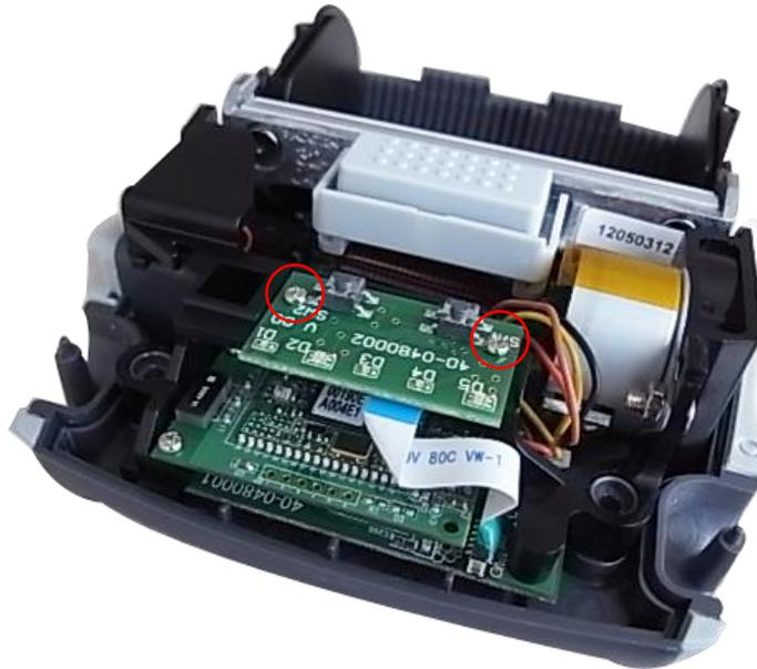
3. Loosen the connector lock then disconnect the flat cable from the keys control board.
