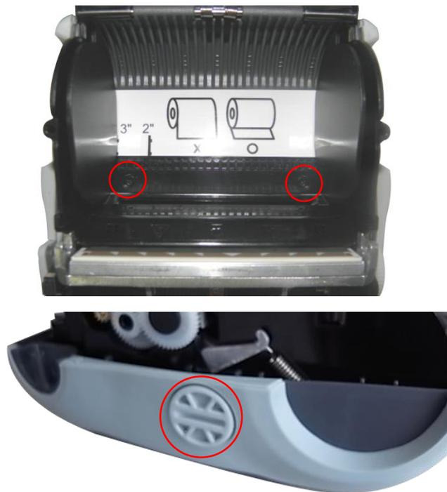
2. Take the interior mechanism from the printer bottom cover.
