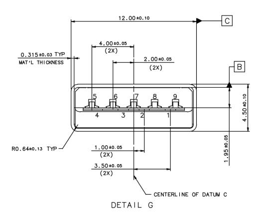
USB 3.0 Standard-A Plug Pin Assignment
