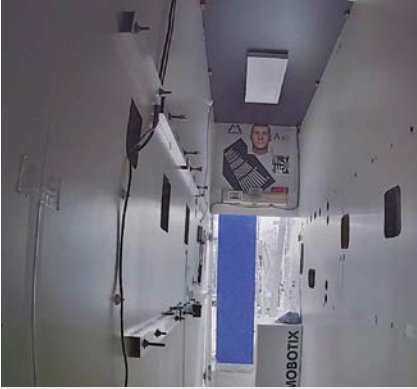
Original MOBOTIX MOVE camera image with activated WDR function: Details are easily recognizable within the dark testing room as well as at the open door with bright light entering through it. The camera automatically combines two differently lit individual images taken within a minimal time difference, thereby forming a live complete image.
