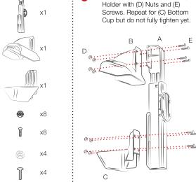
Attach (B) Top Cup to (A) Body Holder with (D) Nuts and (E)
