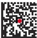
Figure 3-9 DS36X8-DP and DS36X8-DPA Aiming Pattern
