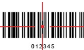
Figure 3-7 DS36X8-HD and DS36X8-HP Aiming Pattern
