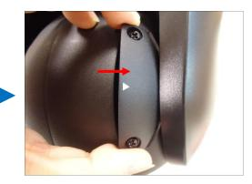
5. Tighten the two (2) screws to secure the cover.
