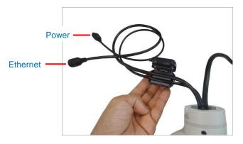
3. Snap the ferrite core to secure it on the cable.
