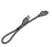
Power cord (Black) - 2-wire, 17 AWG, 0.5m (1.6ft) long - Has straight (F) C7 receptacle (For 240V in UK, Singapore, Malaysia, and Hong Kong, Opt. 955) HP 8121-0893. Cable length: 0.5 m, Connector 2: C7 coupler
