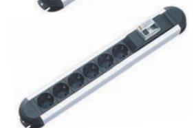
**Overvoltage protection with filter:** Overvoltage protection - conforms to DIN VDE 0620-1:01-2002, EN 61643-11:08-2007, type 3, discharge current 6.5 kA, response time < 25 nS. Suitable for 16A (miniature fuse on request) with varistors, temperature fuse, gas discharge arrester, visual LED function and failure indicator (acoustic signalling also available on request). Mains and frequency filters - conforming to VDE 0565-3:05-2006 for voltage peaks up to 30 MHz, damping diagram on data sheet.
