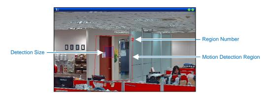
The detection size box indicates the minimum size of the object to be identified as an "object". This feature is useful to avoid false alarms. For example, if the detection size is set to be the size of a human or vehicle, motion detection will not be triggered even when a cat passes the motion detection area.
