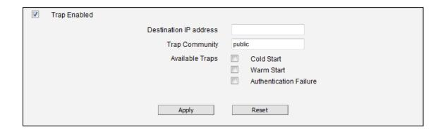
SNMP traps enable notifications from devices. Devices may send message to the management server whenever significant events occur such as cold start, warm start and authentication failure. The manager will get the information immediately and take action if necessary.
