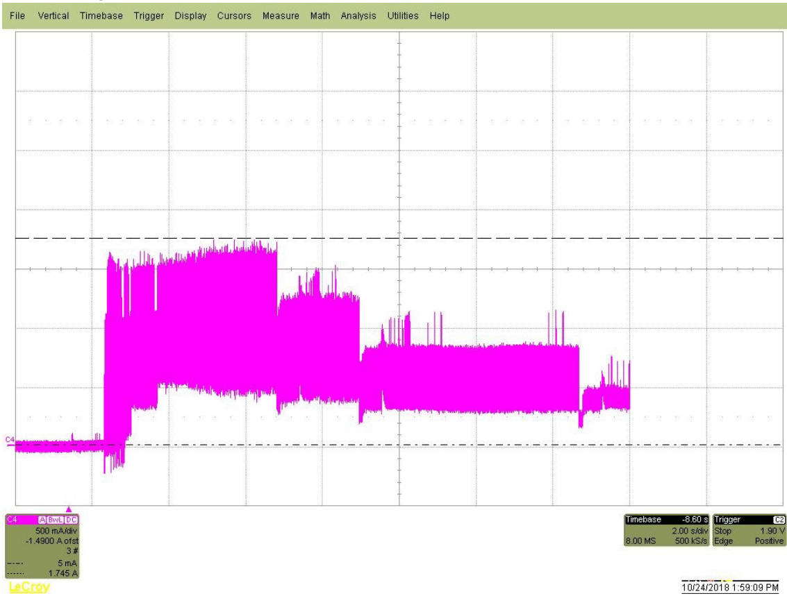
Figure 1. Typical 12V startup and operation current profile
