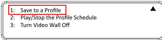
2. To save the active connection configuration as a profile use the front panel number pushbuttons to select a profile into which you want to save the configuration.
