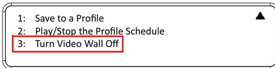
Selecting **Turn Video Wall Off** will return port assignments to their default (i.e. disassemble the video wall).
