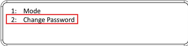
2. In the Old Password field, the cursor flashes at the first digit. Enter the old password (see *LCD Password*, page 42). If the old password is entered correctly, you can proceed to the next step. The default password is: **1234**.
