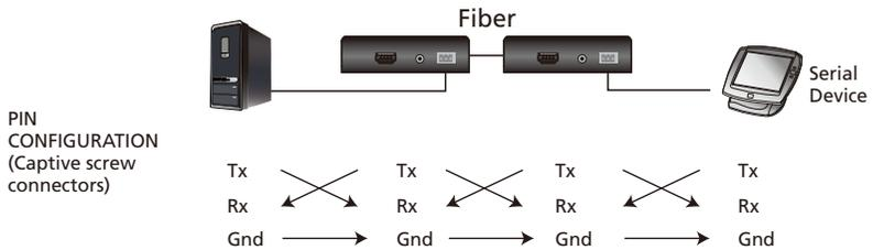
From a source device, the RS-232 signals is transmitted (Tx) to the VE1830 receiving (Rx) unit; the VE1830R transmits (Tx) signals to the display device (Rx).
