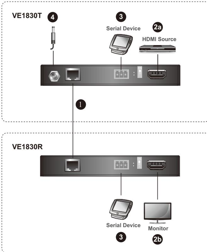
1. Connect one end of a Cat 6a/ATEN 2L-2910 cable to the HDBaseT Out port on the VE1830T and the other end to the HDBaseT In port on the VE1830R.
