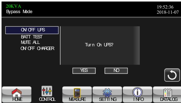
TURN ON UPS
