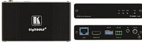
TP-583R is a high-performance, long-reach HDBaseT receiver for 4K HDR HDMI, RS-232 and IR signals over twisted pair. TP-583R converts the HDBaseT signal and outputs it to its HDMI and control ports. It enables extending video signals to up to 70m (230ft) over Kramer copper cables at up to 4K@60Hz (4:4:4) video resolutions. It is compatible with standard HDBaseT-compliant extenders at 4K@30Hz and HD video resolutions
