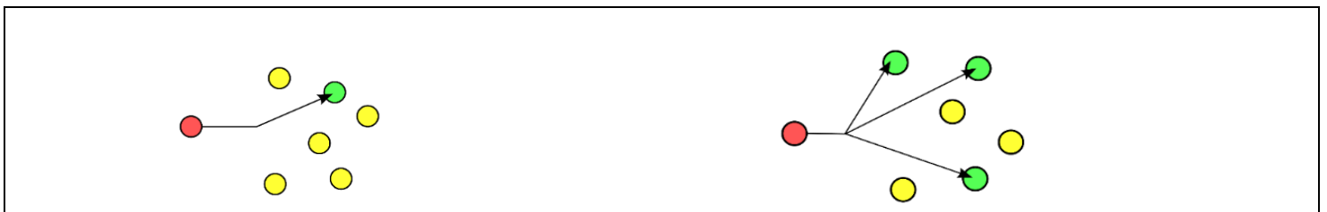
Figure 1: Unicast versus Multicast.
