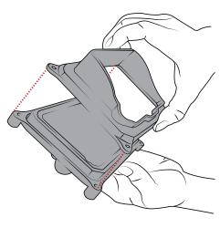
6 Secure all four corners of the cradle assembly using the smaller screws and nuts.
