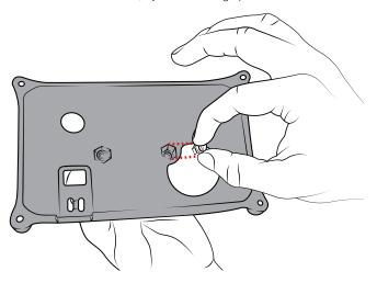
2 Attach diamond ball adapter (not included) using the correct length bolts included in the hardware packet.
