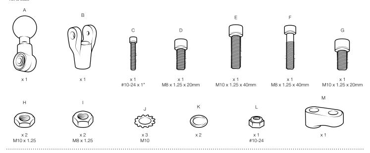
Locate threaded female hole on your motorcycle and verify the appropriate thread pitch by carefully threading one of (D, E, F or G) screws provided. The length of the correct screw will depend on which of the two options you select below. Place correct screw through center opening of (B) clevis base.
