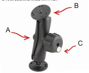
TO ADJUST DOUBLE SOCKET ARM, UNLOCK KNOB (TURN KEY COUNTER-CLOCKWISE) AND LOOSEN BY ROTATING KNOB COUNTER-CLOCKWISE. WHEN DOUBLE SOCKET ARM AND BASES ARE ADJUSTED TO DESIRED POSITION, ROTATE KNOB CLOCKWISE TO TIGHTEN. TO LOCK, TURN KEY CLOCKWISE.
