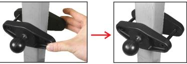
3. Rotate RAM® Clamp Base assembly to reduce any gap between the (C) Screws and the square post. Tighten Screws using 3/16" Allen Hex Key.
