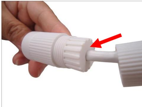
16. Connect the RJ-45 connector to the camera connector.
