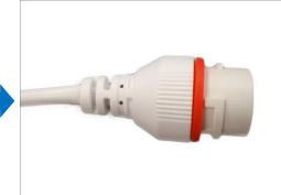
2. Detach the clamping nut and sealing insert from the gland body:
