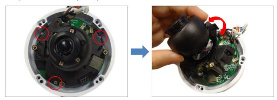
**NOTE:** Do not abruptly lift the camera module, cables are connected underneath.
