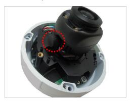
2. Rotate the lens module to change the viewing orientation.
