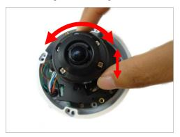
3. Tighten the tilt adjustment screw to fix the lens position.
