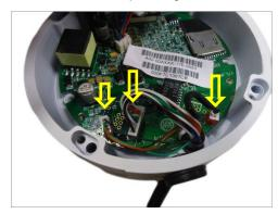
8. Attach the camera module back.
