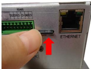
Once inserted, make sure to access the camera Web Configurator and “mount” the card to prepare the card for local recording. Refer to the camera Firmware User’s Manual for more information.
