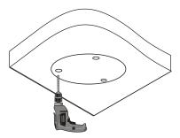
2. Insert the plastic anchors and drill a hole to lead the cables out of the ceiling.
