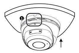
6. Adjust the lens viewing direction, and then tighten the screw.
