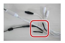
Connect the tail cables, and protect the cables and cable connections using insulating tapes. Then wrap all the tail cables together using insulating tapes.
