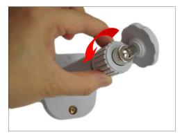
3. Screw the camera to the bracket.
