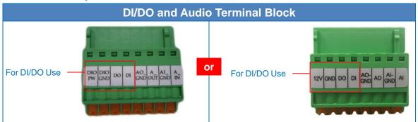
To connect digital input / output devices (DI/DO), map the pins to one of the pin combinations below:
