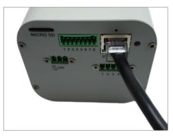
2. If necessary, connect the other external devices, such as DI/DO, PT scanner or power adapter to the camera. See *Before Installation* on page 15 for more information.
