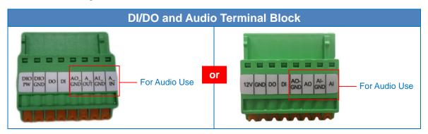
To connect audio devices, map the pins to one of the pin combinations below:
