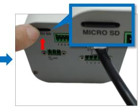
For E210, after inserting the memory card, use the slot cover to close the memory card slot.
