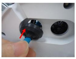
6. Pull enough Ethernet cable length to be able to connect to the Ethernet port of the camera.
