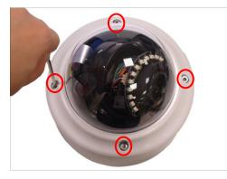
2. Loosen the four (4) screws and detach the base plate from the camera.
