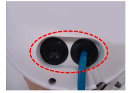
**NOTE:** If no other devices will be connected, make sure that the other rubber is properly placed on the camera cable hole.
