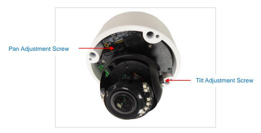
**NOTE:** Be careful when turning the lens module to its extent as cables are connected inside the module.
