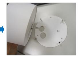
3. Using the drill template, mark the screw holes and cable holes (as needed). Then install the base plate to the wall or ceiling surface using the bundled screws. Take note of the orientation of the camera before you mount the base plate.
